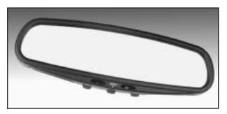
The vehicle may be equipped with an automatic dimming rearview mirror. Push the center button on the bottom of the mirror to turn this feature on. The mirror will darken gradually to reduce glare from headlamps behind you. This may take a few moments. The mirror will lighten whenever you shift to REVERSE (R).
